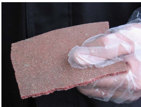
A piece of removed floor covering with PCBs
