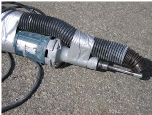
Straight die grinder used where the workarea is difficult to reach. A dust collecting nozzle with an adjustable hose is applied on the die grinder from Bosch (GGS 27LC).
