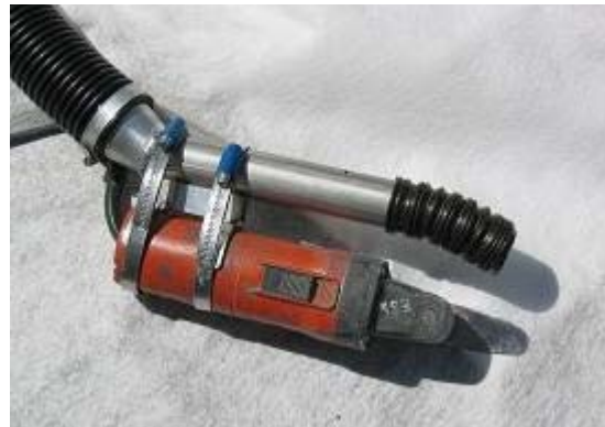
Oscillating knife cutter from Fein, model FSN 400E with the SP dust collector and Riktaflex.
