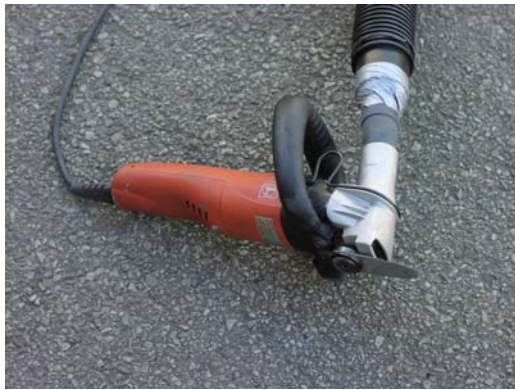
A new oscillating knife cutter from Fein, model FSC 1.6, used to cut out the PCB containing sealant from the joint.
