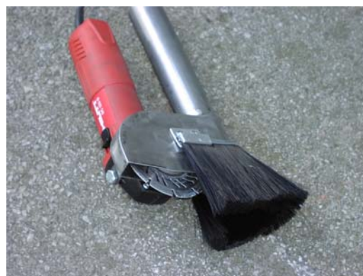
Grinder from Hilti (DC 125-S/EX) with cutting disc for sawing in concrete, with the new SP dust collector.
