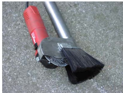
Grinder from Hilti (DC 125-S/EX) with cutting disc for sawing in concrete, with the new SP dust collector.
